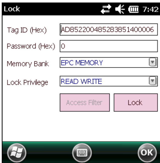
Figure 4-18 Lock Access Operation Window
