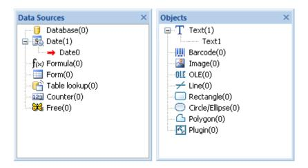
The up and down arrow keys on your keyboard allow you to move up and down the object tree. The + and - symbols allow you to expand or shrink the list and display the list of variables associated with each data source or the objects available for each category.
